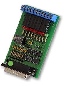
The control information from the software "PCLOG " or "PROFILAB" is transferred over the PC LPT-Port as a binary signal. The relay cards supplied as accessories are needed to connect power devices like heaters, valves, servomotors or alarm buzzers. The switching status is indicated with LED's. The relay boards are also used for many other applications.
