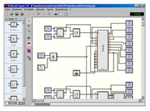
With this software, professional measurement and control projects can be realized in a simple, graphics based development platform. You can simply draw the wiring diagram of the measurement circuit and do the project design. Without any knowledge of programming, the measurement values of up to 16 temperature sensors can be easily used in the measurement circuit.
